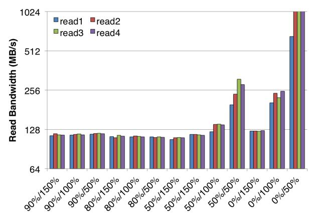
The above diagram shows the measured bandwidth from a single node with 128 GiB of total DRAM. The first percent on each x-label is the amount of this 128 GiB that was reserved by the benchmark as application memory, and the second percent is the total write volume. For example, the "50%/150%" data points correspond to 50% of the node memory (64 GiB) being allocated for the application, and a total of 192 GiB of data being read.
